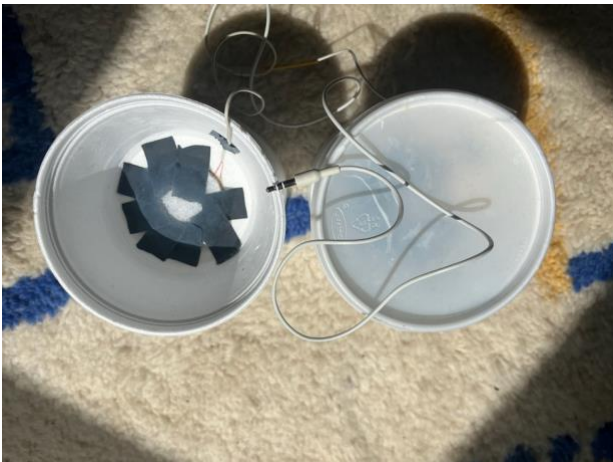
Figure 11: Styrofoam takeaway container microphones
