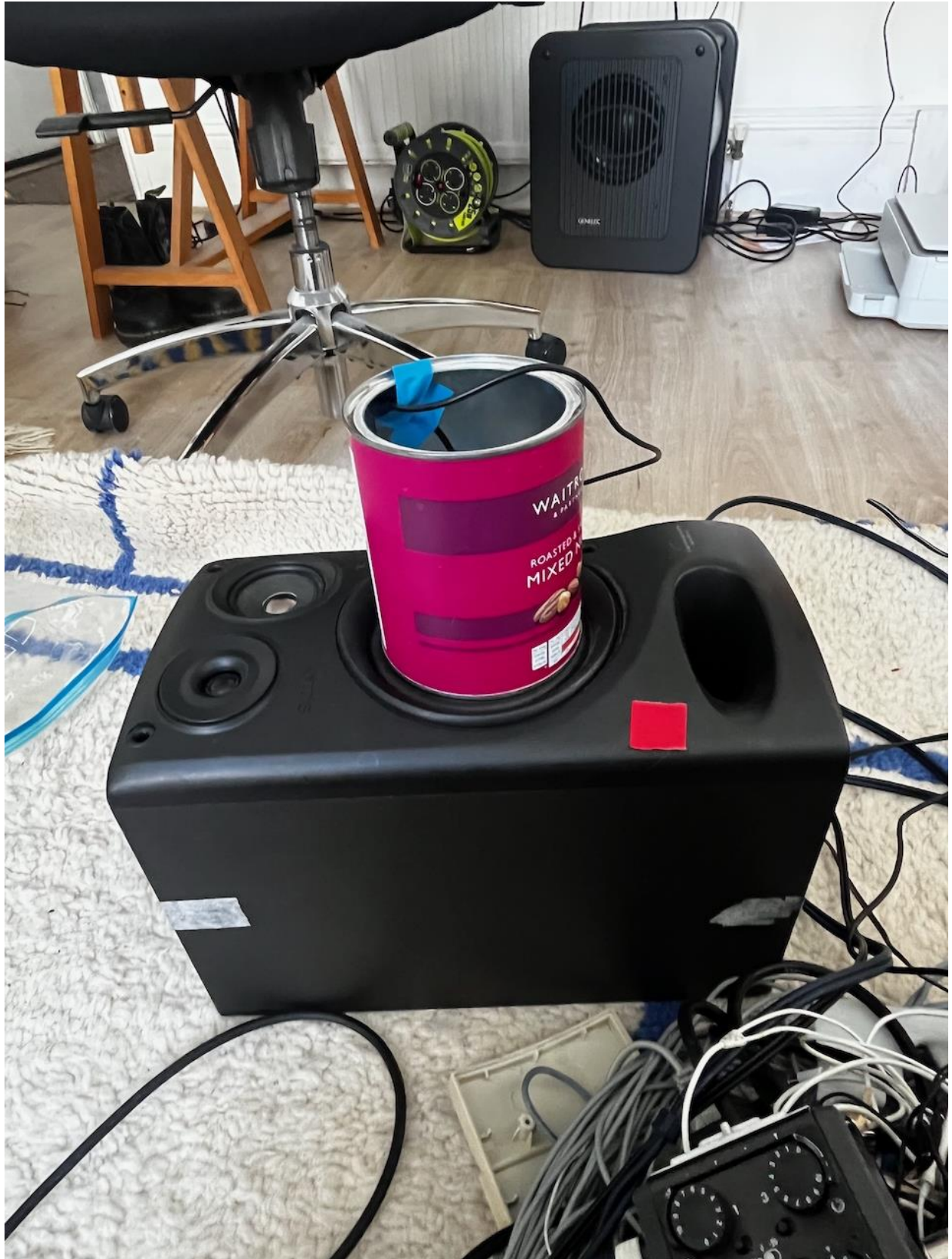
Figure 8: Modulation of sound on 5" speaker cone with a homemade WEEE microphone
