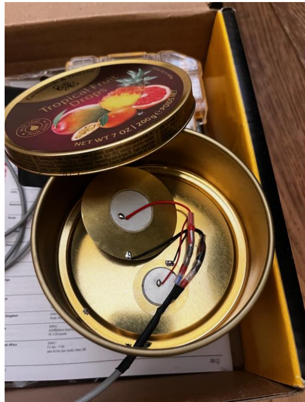
Figure 12: Candy "tin" unknown alloy, piezo
